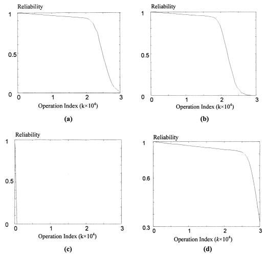
Figure 11. Impact of fixture layouts on fixture-system reliability using different threshold methods: (a) method 1 using  $P_1$ ; (b) method 1 using  $P'_1$ ; (c) method 1 using  $P''_1$ ; (d) method 2 using  $P_1$ ,  $P'_1$  and  $P''_1$
