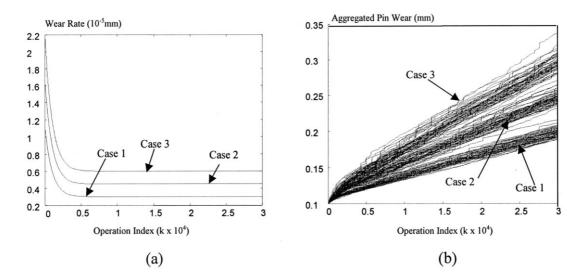
Figure 13. Comparison of the aggregated wears under different wear parameters: (a) different pin-wear parameters; (b) aggregated pin wear
