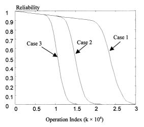
Figure 14. The effect of component wear rates on fixture-system reliability
