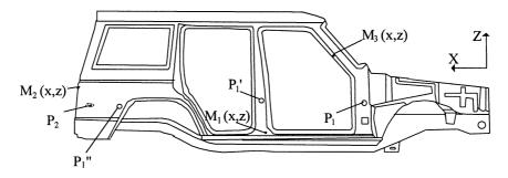
Figure 6. Layout of the fixtures and KPC points
