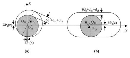
Figure 3. Locating error due to fixture system component wear: (a) four-way locating pin  $P_1$ ; (b) two-way locating pin  $P_2$
