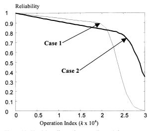
Figure 15. The joint effects of part quality and fixture-system component catastrophic failures
