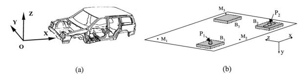
Figure 2. Automotive body and its assembly fixture: (a) body coordinate system; (b) 3-2-1 fixturing principle for rigid part
