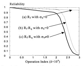
Figure 9. Fixture-system reliability analysis with and without considering the QR-Co-effect
