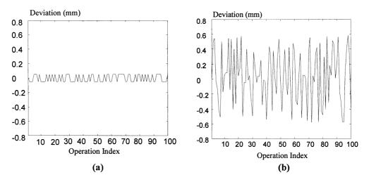
Figure 12. Comparison of part-locating error with KPC deviation: (a) early stage deviation at pin  $P_1''$ ; (b) early stage deviation at  $M_3$
