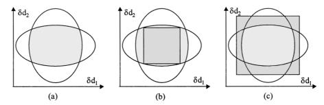
Figure 10. Comparison of KPC constraints and tool wear contraints: (a) quality constraint on KPC; (b) over-constraint on pin wear; (c) underconstraint on pin wear
