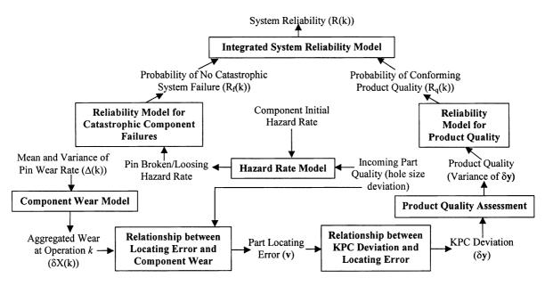
Figure 5. Summary of the QR-Co-Effect model for a fixture system
