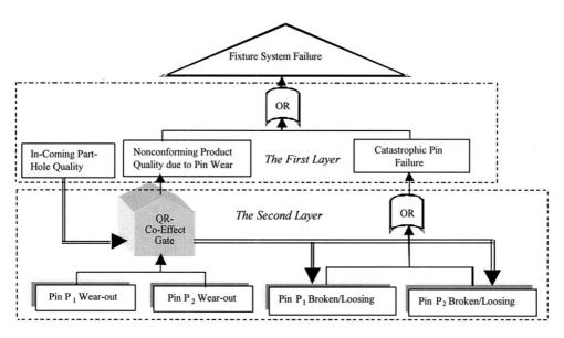
Figure 4. Fault tree analysis of a fixture system
