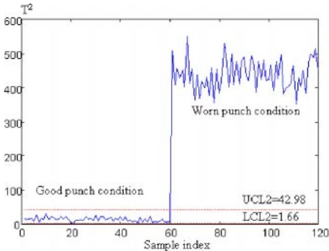
Fig. 7 Phase II control limits to detect the out-of-control condition
