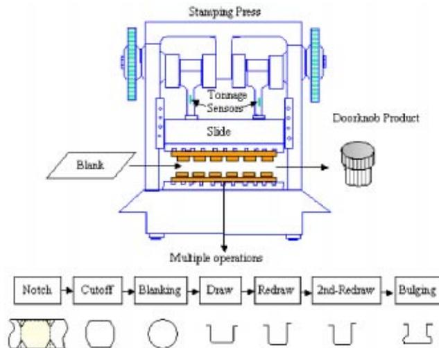
Fig. 3 Multiple operations in the doorknob stamping process
