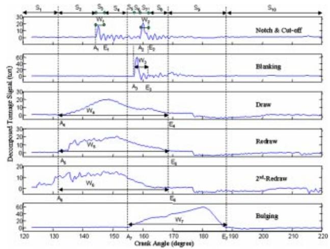
Fig. 4 The decomposed individual signals at each working station
