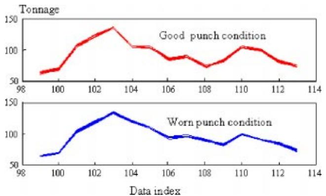
Fig. 5 Press tonnage signals at two different punch conditions
