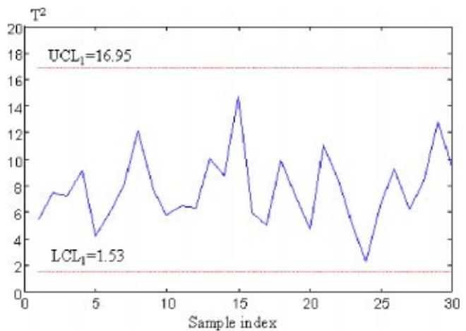
Fig. 6 Phase I control limits to check the preliminary in-control data
