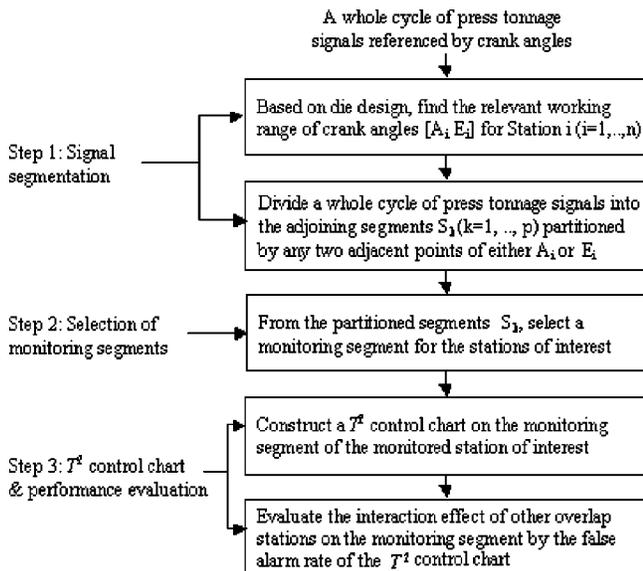
**Fig. 1 Analysis framework for multiple-operation stamping process monitoring**
