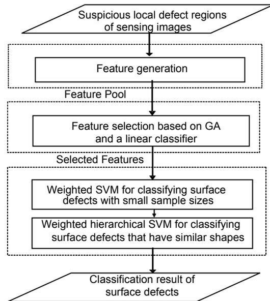
FIGURE 2. METHODOLOGY OF CLASSIFICATION METHOD BASED ON SUSPICIOUS DEFECT REGIONS OF SENSING IMAGES.
