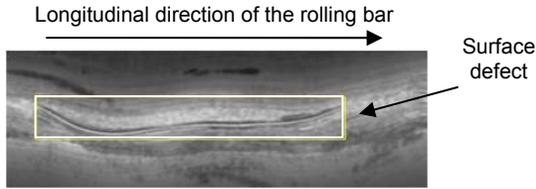
FIGURE 1. REAL TIME SENSING IMAGE OF A HOT BAR IN A ROLLING PROCESS
